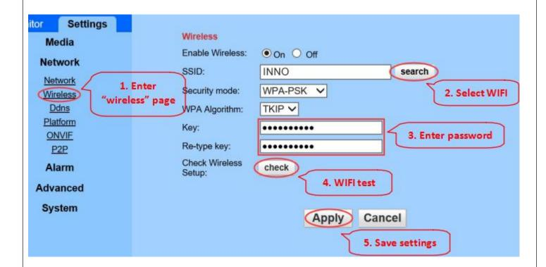
The WIFI connected to the camera must have a signal value greater then 50% and WIFI name must be english and can not contain special characters.
